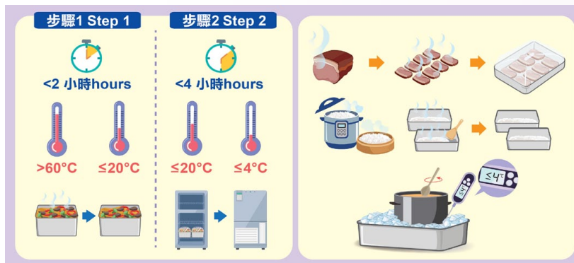
圖2: 二段冷卻法和加快冷卻的技巧 Figure 2: Two-Step Cooling Approach and Techniques of Speeding up Cooling
