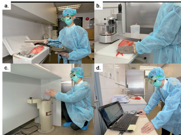
(a) 利用手提裝置檢測輻射水平。(b)至(d) 準備食物樣本並利用污染監測系統檢測樣本中各種放射性核素的含量。 (a) Detection of radioactivity level by hand-held device. (b) - (d) Sample preparation and detection of activity of different radionuclides in foodstuffs with Contamination Monitoring System.
